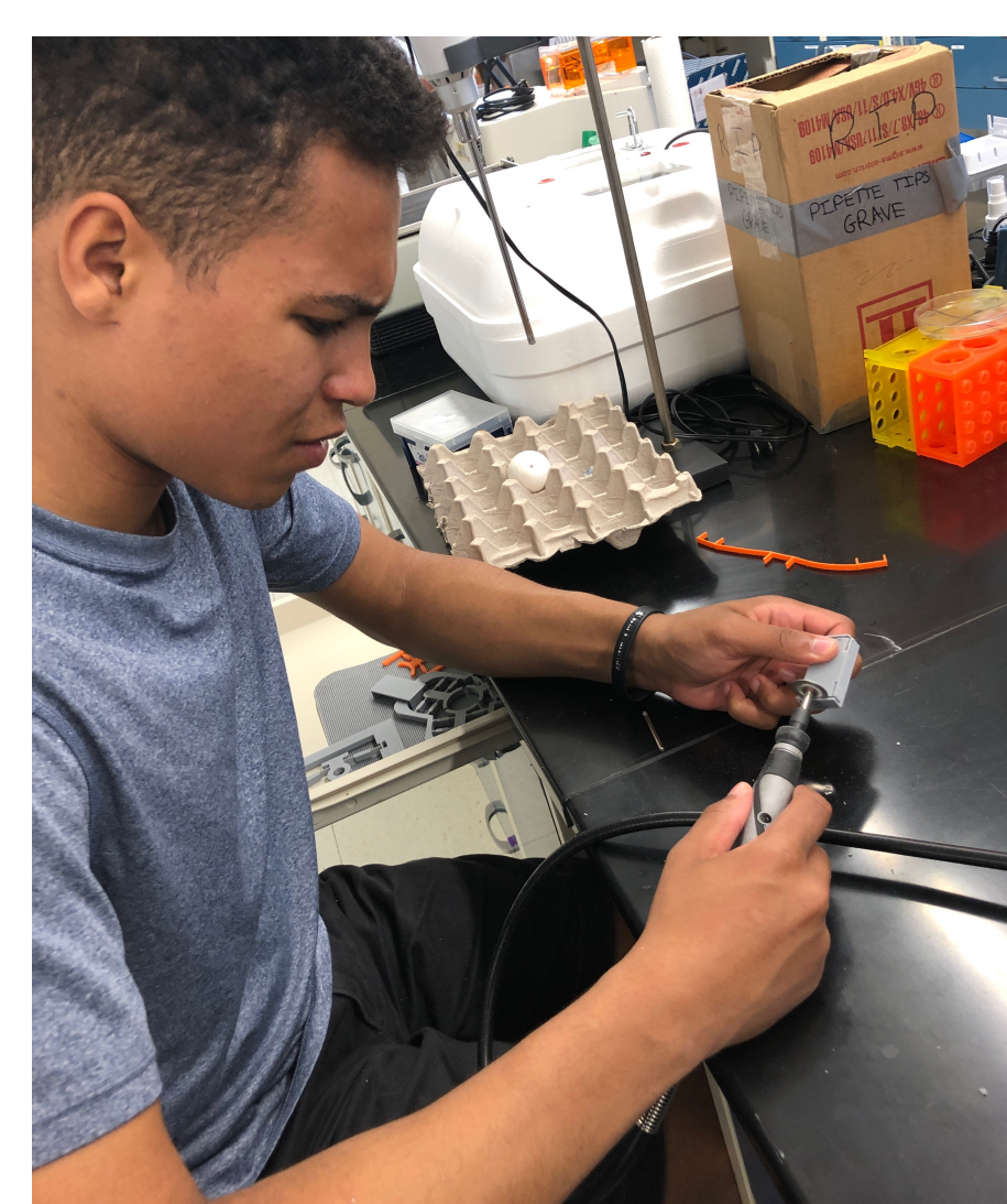
Using Dremel to modify fit of 3D print
